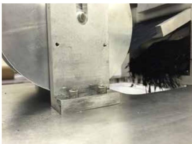
**Figure 9.** Digital photograph of the continuous extraction process for CNTs grown on the surface of a metal foil. The CNTs have greater than 99% purity and will not require any additional purification process.
