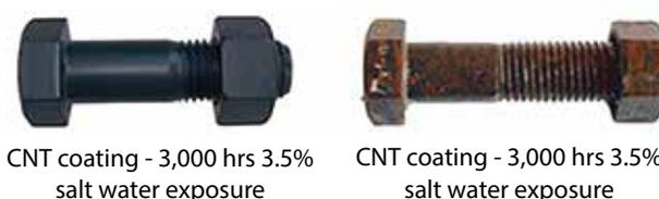
**Figure 15.** Digital photographs showing CNT coating of metal nut and bolt in preventing oxidation when exposed to high concentration salt water.
